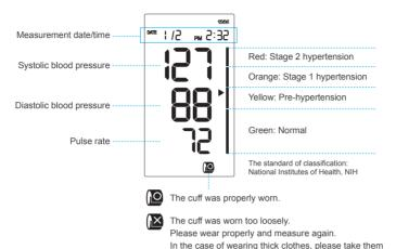
2 Check for Morning Surge Hypertension, Irregular heartbeat and Detected Motion. The user can know the blood pressure values or peculiar items of the measurement through icons in the lower part of the blood pressure monitor screen.
